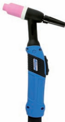
TBi SR 400 100% (10 min.) AC: 400 A DC: 450 A Ø 0.5-4.8 mm
